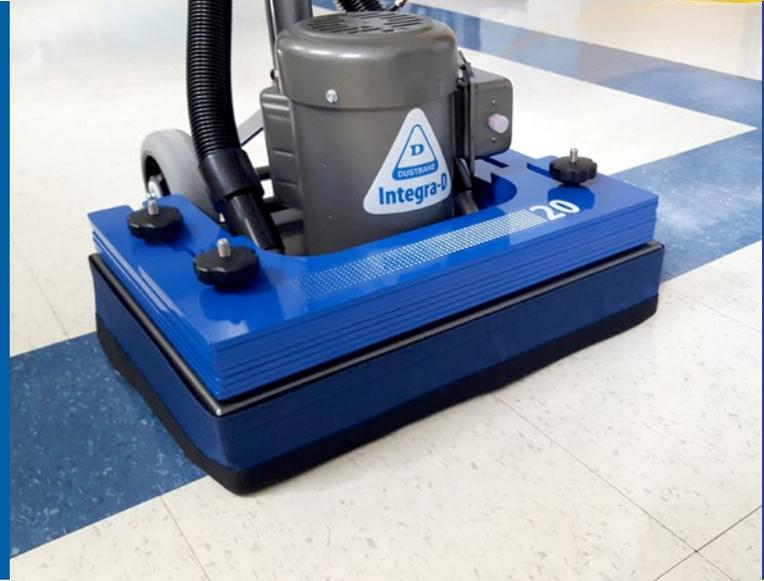
A uniquely designed floating head completely eliminates any vibrations through the handle – preventing directional drift and making steering effortless.
