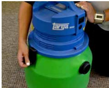
2. Attach swivel connector of suction hose to inlet nozzle on tank.
