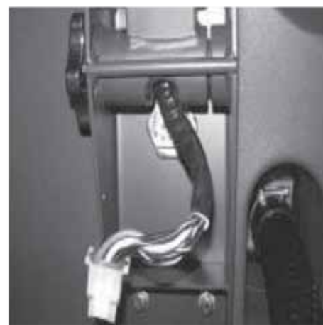
6. Attach the wire harness to the machine.
