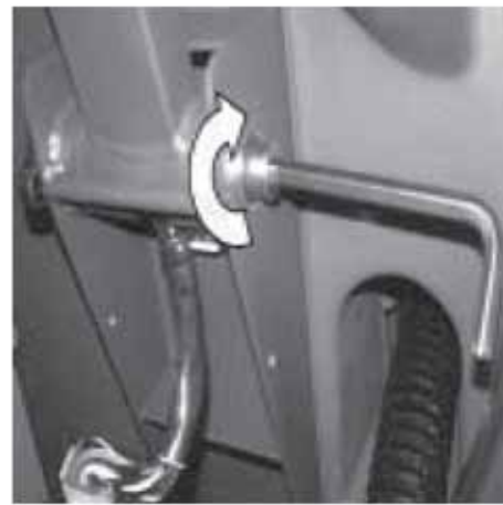
3. Insert handle assembly in between bushings. Insert the shoulder bolt through the bushing and screw into the handle assembly using supplied wrench.
