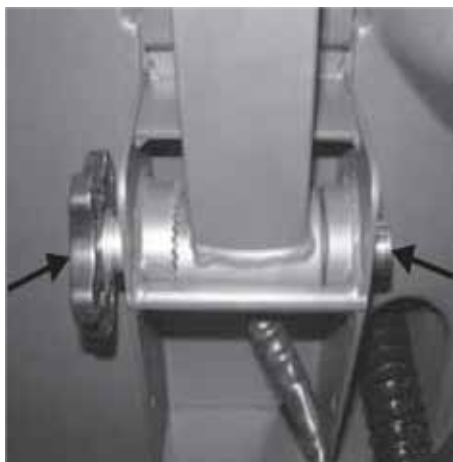
4. Align the teeth on the bushing and handle assembly before tightening the adjustment knob.
