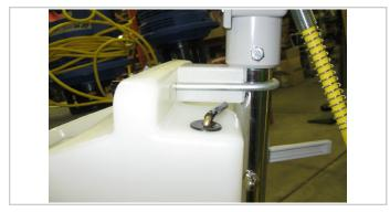
1. Attach U-Bolts to handle with block as shown. Upper U-Bolts should be tight to switch box.
